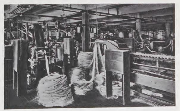
An intermediate step in the combing process. After their final working these "slivers" are transferred to the spinning department, where they are reduced in size by an additional combing and drawing operation, after which they are twisted into yarns.
