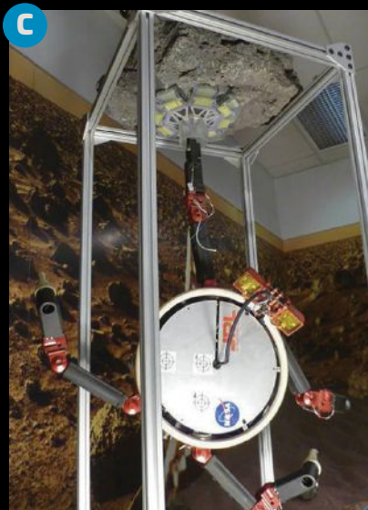
LEMUR IIb climbing robot using a bioinspired gripper to hang from a model Martian rock.
