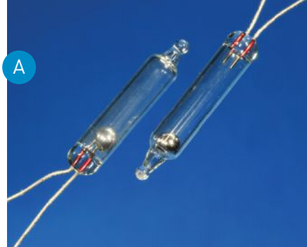
A blob of liquid mercury makes a connection between two contacts (left) or leaves them exposed (right) depending on the angle of the glass capsule.
