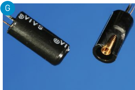
A vibration sensor (left) is cut open (right) to show the tiny rod and spring inside.
