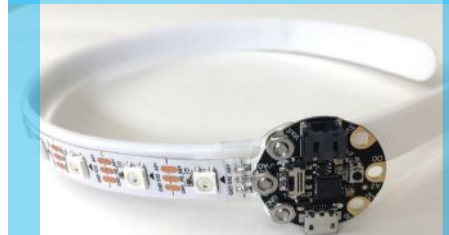
Headband guts: Gemma M0 and an LED strip
