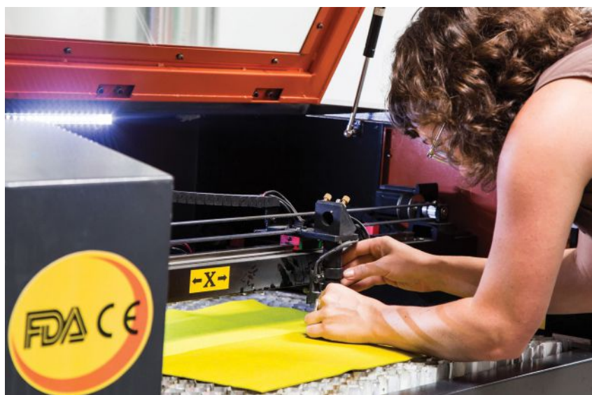
Laser cutters can cut, etch, or engrave a wide variety of materials, such as fabric, plastic, and glass.
