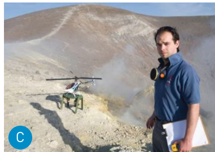
Andrew McGonigle and his remotely controlled copter for sampling the air over active volcanoes.
