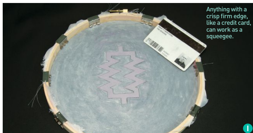
Paint the resist over all areas where ink should not pass.
