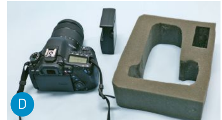
A coping saw can cut holes for equipment such as a camera and battery charger.
