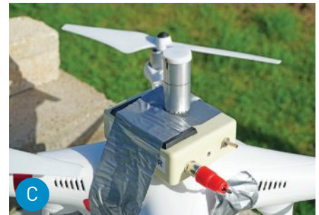
A UV-B radiometer taped atop a Phantom 3.
