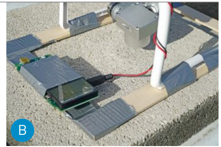
An Onset 16-bit data logger taped to a drone instrument platform.
