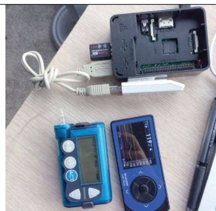
Early OpenAPS rig with an insulin pump, continuous glucose monitor, and Carelink USB stick.
