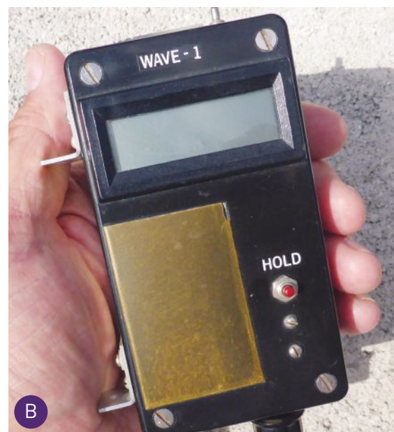
Near-infrared hygrometer used on the Chicago flight whose captain choked me.
