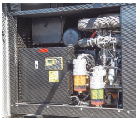
A PowerTech 50kW generator serves up to 200 amps on the Red Triangle Coffee + Provisions truck.
