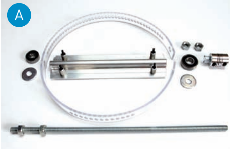
The mechanics: bent and drilled polycarbonate rotor, ball bearings, M8 threaded rod, aluminum flanged tube, flexible shaft coupling, and fasteners.
