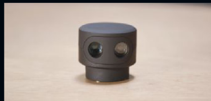
The Sweep lidar unit from Scanse, a $250 single-laser device that rotates 360° to map a single plane of an area.
