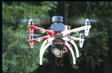
Roughly the size of a hockey puck, and just over a quarter pound in weight, Sweep is one of a few new lidar devices that hobbyists can access for experiments like aerial drone mapping.
