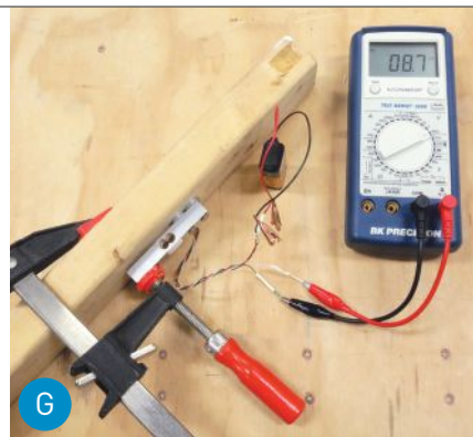
Figure G: Use a screw clamp to calibrate the Grip Challenge.
