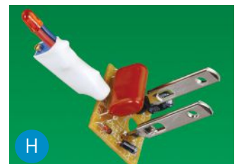
Heat-shrink tubing insulates the new LED assembly.
