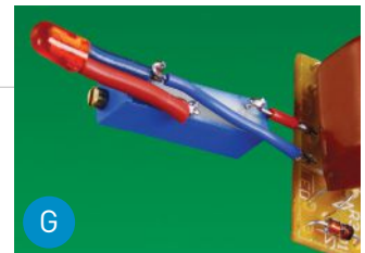
The LED and trimmer soldered to the output from the board.
