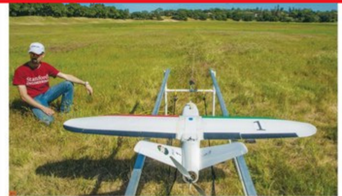
Michael Taylor, with Uplift Aeronautics' Waliid drone mounted on a home-built PVC launcher
