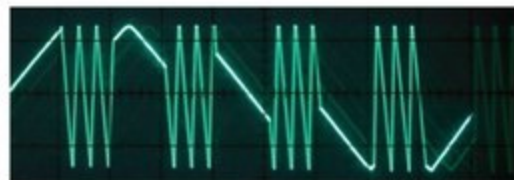
D Move switch 5 down: the 7555 output makes the XR2206 alternate between 2 frequencies set by 500K trimmers.
