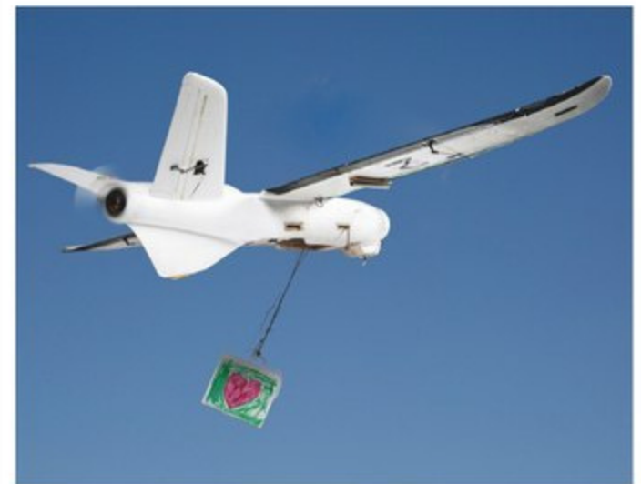
When the cargo bay releases a shipment, the weight of the box pulls a parachute, made from plastic bags, out of the drone
