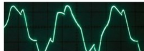
F Applying the 7555 timer output to pin 7 of the XR2206 chip produces unpredictable results.
