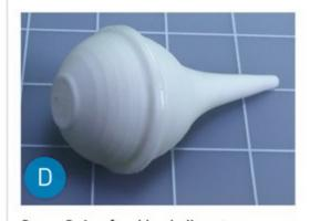
Figure D. A soft rubber bulb syringe, intended for the nostrils of infants, makes for an impressive pushbutton.
