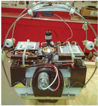
Inside is a mix of repurposed materials, including hard drives, cutting boards, brush handles, and two Power Wheels motors.
