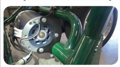
3-phase AC motor attached to swing arm.
