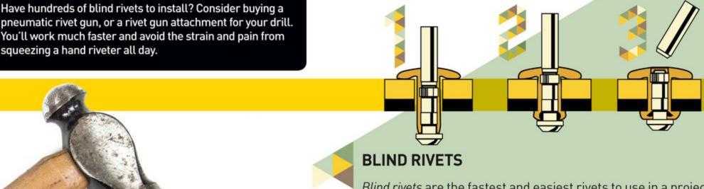
Blind rivets are the fastest and easiest rivets to use in a project. Often called "pop" rivets (after a popular rivet brand), they can be installed completely from one side, unlike solid rivets or bolts that require access to both sides of the material. If set correctly, blind rivets produce reliable fastenings without all the hammering involved in solid rivet installation.
