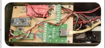
The electrical deck of Chibi-Mikuvan: an Arduino Nano, a modified USB charger as power supply, a highcurrent relay between battery and motor controller, and a current sensor. The red component is a backup logic power supply.
