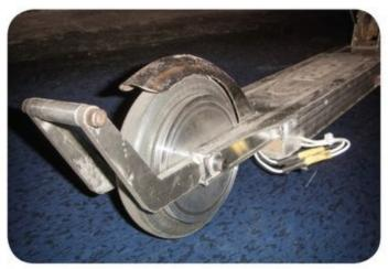
A small "hub motor" scooter I built in 2008 that I used as transport for 2 years.
