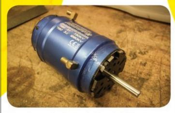
This soda can-sized motor for 1/5 scale R/C boats can output several thousand watts of power — but it spins at over 20,000rpm to do so.
