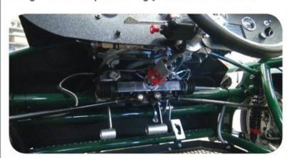
Under the dash: dual brake pedals, steering linkages, and accelerator — step on it, but don't call it a gas pedal.
