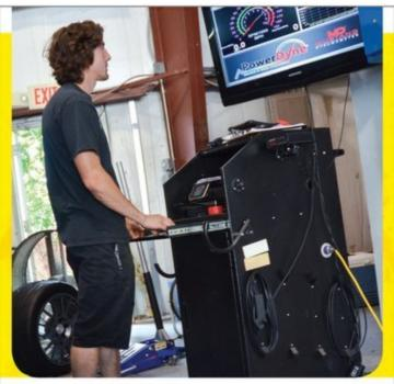
Hogarty at the console of a dynamometer, which allows him to verify how changes to an ECU affect torque and horsepower.
