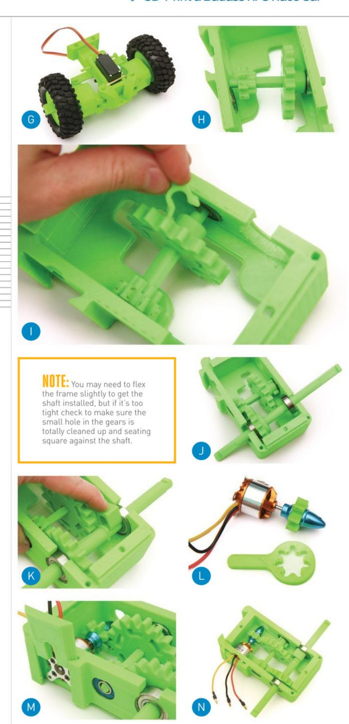
wheel assemblies using the short and long pins.
