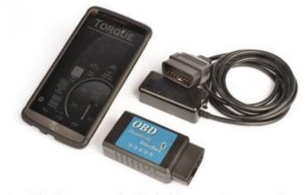
The Torque app for Android accesses your car's OBD-II port to track engine data and display it on your smartphone.
