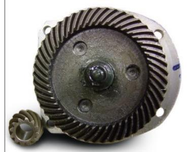
The insides of an inexpensive imported 9" handheld angle grinder's gearbox.
