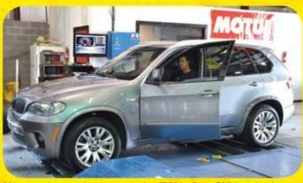
Hogarty tests changes to the ECU of an SUV as it sits on a dynamometer.
