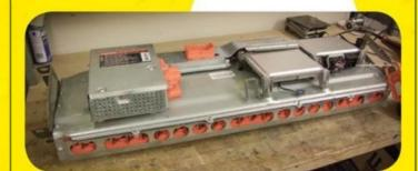
A hybrid car battery module, made of many smaller low-voltage cells which can be reconfigured.
