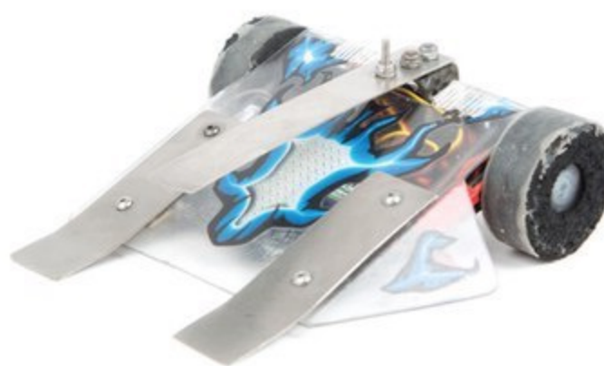
Micro Drive, Zachary Lytle's original champion, is a scale model of his full-size competition fighting robot, Over Drive.
