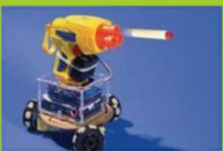
R/C OMNIWHEEL ROBOT An easy holonomic "Kiwi drive" robot that moves instantly in any direction.
