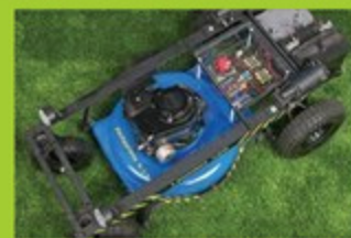
LAWNBOT 400 Hate mowing the lawn? Make an Arduino-controlled R/C lawnmower!
