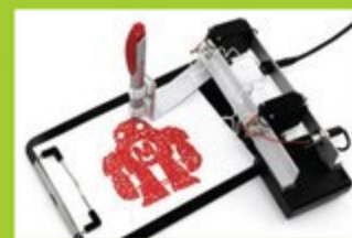
TRS DRAWBOT Turn tunes into 'toons with a robot arm controlled via headphone jack.
