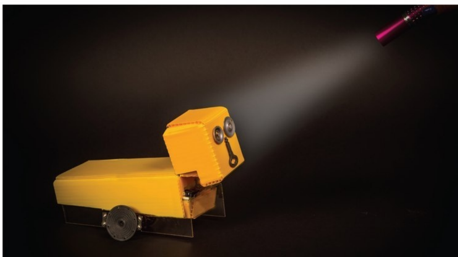
Figure I: Each servo is bolted into a notch cut in the frame. The wheels were included with the servo recommended for this project.
