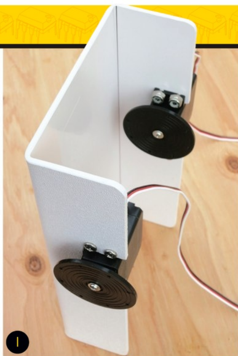
Figure I: Each servo is bolted into a notch cut in the frame. The wheels were included with the servo recommended for this project.
