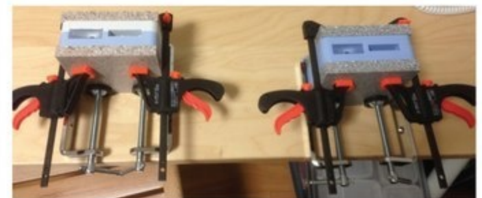
Preparing an early version of the Edison for resin encapsulation using silicone molds. The method was used in lieu of standard cases. Polishing the resin made it possible to see the internals.
