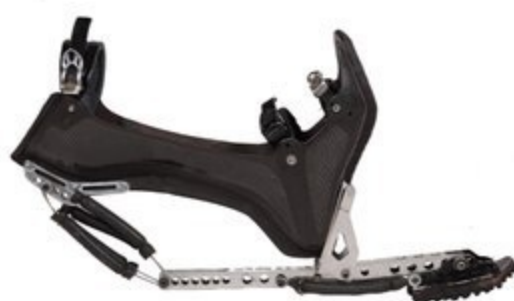
X11-2011 — First fully carbon-fiber exoskeleton, molded to encompass the anatomy of my leg. The shape transmits the force in the boot as the main lever stretches the spring.
