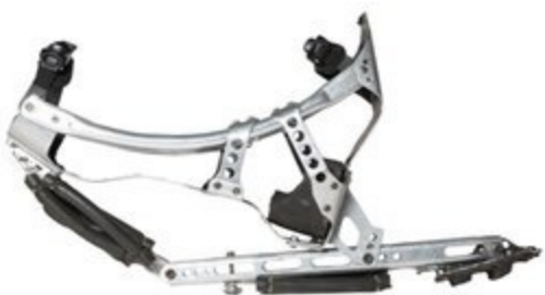
X10 (rev.)-2010 — Altered the exoskeleton shape. More advanced structure doesn't use aluminum tubes for main support — the sculpted metal provides the strength.
