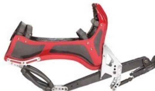
X12- 2012 — A carbon-fiber lever and toe reduced weight but failed due to the high forces involved when running. Double toe increased mobility on uneven terrain.
