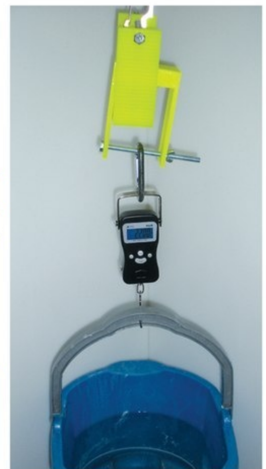
Crush test setup, post-crush.
