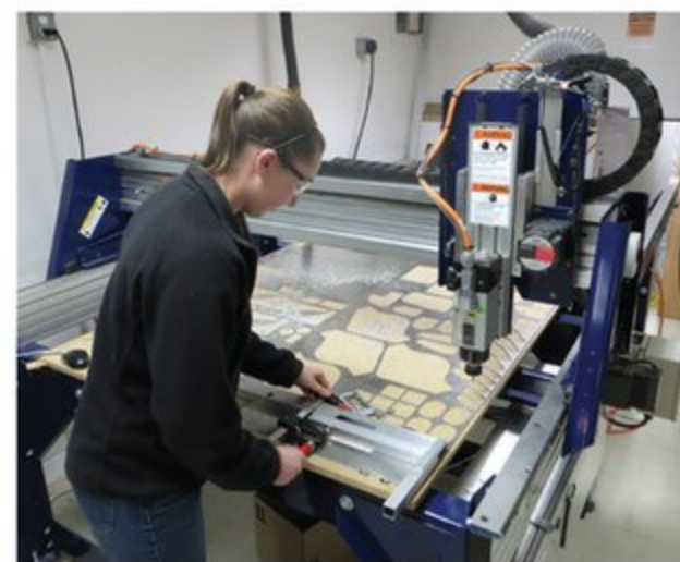
TEC Hub student cuts aluminum robot parts on full size ShopBot
