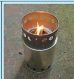
WOOD GAS CAMP STOVE Make a simple tin-can stove that runs for free and even sequesters carbon as you cook.
