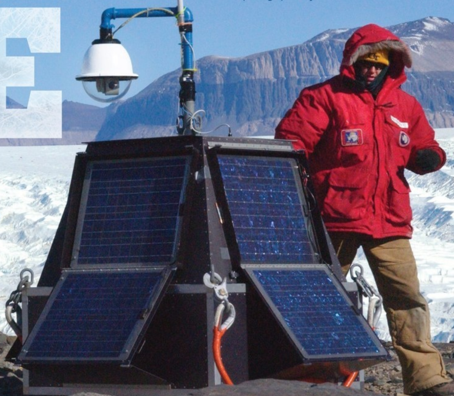
POLAR SOLAR: The team's TAISU carbon-sensing device, with wi-fi observation camera, at the top of the Bonney Riegel in the Antarctic Dry Valleys.
