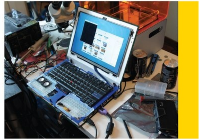
A DIY laptop parked in front of the Form 1 3D printer used to make its body panels.
