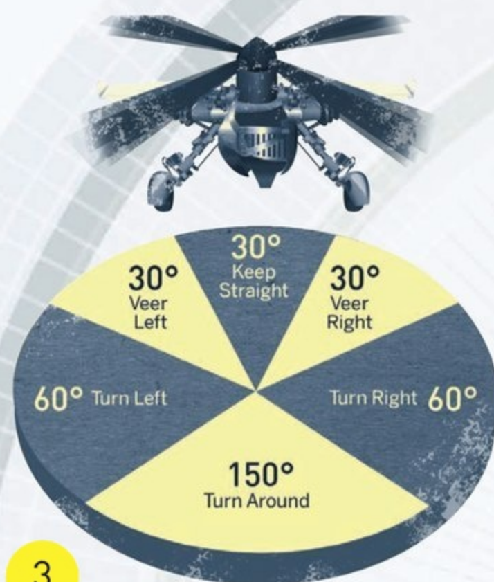
How FindingYourself.ino translates your course and bearing into text directions. The sketch can become the starting point for creating almost any type of autonomous or semi-autonomous vehicle.
