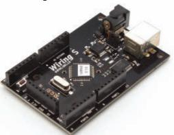
factor so you can reuse your Arduino shields with your Wiring boards.
