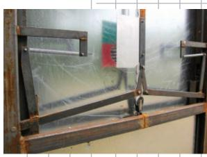
CAT'S CRADLE: Prototyping a mechanism like the tiger gate is a combination of the usual R&D and collaboration with the zookeepers, who are experts in animal behavior. Many pulleys, counterweights, and trials by zookeepers led to the final design.
