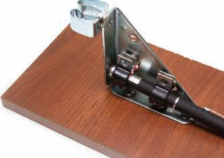
Mount the laser in its 2 clips and attach them to the triangular vertical plate. Then align the lens with one of the holes in the upright. Add washers between the magnet and the clamp if necessary to adjust spacing.
