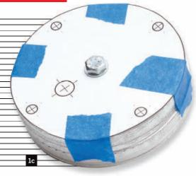
(**Figure 1c**). Center-punch all holes (**Figure 1d**) and remove the template.
