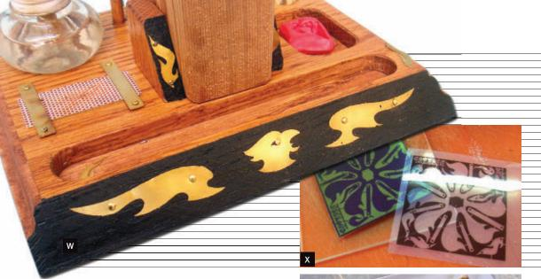
leaving an acid-resistant pattern. Place it in ferric chloride solution to etch away the unprotected areas, leaving your brass part (Figure Y). I used Micro-Mark's terrific all-inone etching kit, which comes with complete instructions. (Watch for a future article on that!)
