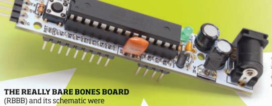
originally designed by Paul Badger of Modern Device. It's pretty much the bare minimum needed for a useful Arduino-type development board. And once you build the schematic in EAGLE, it's easy to incorporate in
