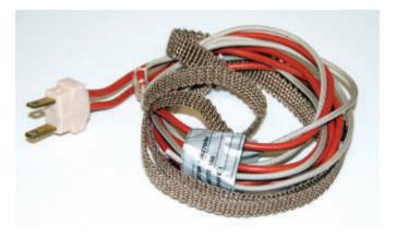
weave; the electrical plug is split, with the power lead at one end of the strip and ground at the other, which avoids having to use pricey heatproof insulation on the return wire. The BriskHeat can bend plastics up to ½" thick, quickly and cleanly — a fact anyone who's ever tried doing it with a heat gun will appreciate.
