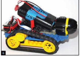
host computer, because it is able to emulate a keyboard, mouse, joystick, or send data directly. One of the more complex and memorable standalone projects built with the Digispark is the CamBot by Dave Astolfo. The CamBot is a Bluetooth-controlled robot built from Legos, a Digispark, a Digispark Motor
