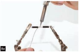
1/4" of insulation off the ends, and bend each wire into an S shape. Solder one wire to each free end of the diodes and the third wire to the joint between the two (**Figure 8b**). Crimp a ring terminal to the free end of each of the 3 wires (**Figure 8c**).
