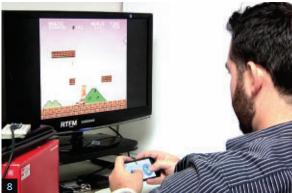
puter. (The BLEduino app is a really important aspect of our board since it provides all of the UI and libraries necessary to communicate with the BLEduino.) The BLEduino creates the keystrokes by simulating a normal keyboard hooked up to the computer via the USB port and receives the commands via BLE.
