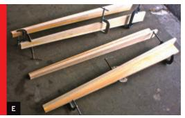
To make the finished legs symmetrical when the pairs are butted together, I chose 4 of the 8 pieces and ripped 34" off the untapered edge. This left 4 pairs of tapered boards, 2 for each leg: one measuring 31/2" wide at the untapered end and the other measuring 23/4".
