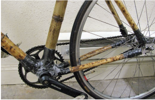
HAULING GRASS: (Clockwise from top left) The prepared bamboo, oven-cured, torch-hardened, and ready to make frames; a bamboo bike rack by Boo Bicycles; the personal ride of a Bamboo Bike Studio co-owner; and a close-up of its hardware connecting the bamboo chain stays, seat stays, seat tube, and down tube.
