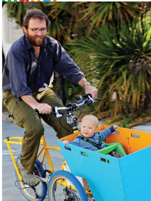
TYKE LIKE TRIKE: Saul Griffith carries his young son, Huck, in an early prototype of his cargo trike. The triangular wheelbase and innovative tilt-steering system ensure that the trike stays safely upright while it's stopped, traveling in a straight line, or turning at any normal radius and speed.
