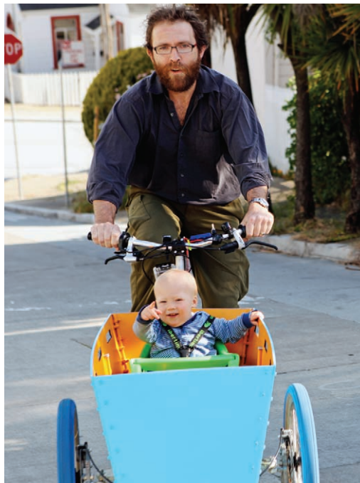
TYKE LIKE TRIKE: Saul Griffith carries his young son, Huck, in an early prototype of his cargo trike. The triangular wheelbase and innovative tilt-steering system ensure that the trike stays safely upright while it's stopped, traveling in a straight line, or turning at any normal radius and speed.
