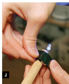
Fig. I: Run the secondary motor wires through the U channel. Figs. J and K: Tape a glowing LED to the end of the secondary arm, then start experimenting with long-exposure photos.
