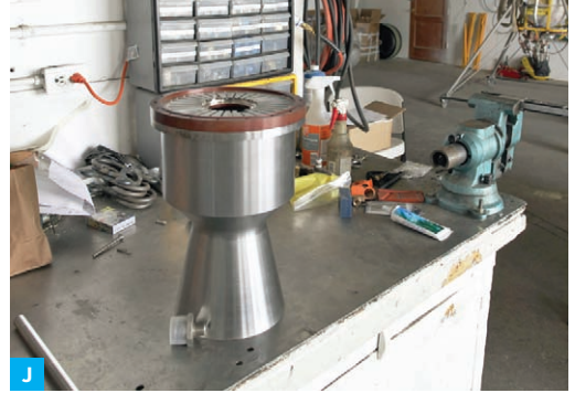
Fig. I: Dick Rutan works on his Berkut, a kit-built aircraft descended from the Long-EZ design developed by his brother, Burt. Fig. J: A rocket motor stands on a workbench in a Masten Space Systems hangar at the Mojave Air and Space Port. The motor was turned from a block of aluminum at a local metal-fabrication shop. It is double-walled, enabling circulation of coolant to prevent the aluminum from melting. Fig. K: The XA-0.1-B (generally known as Xombie) won second place in Level 1 of the NASA-funded Northrop Grumman Lunar Lander X Prize Challenge in 2009. Xombie is still being used for flight testing new systems.
