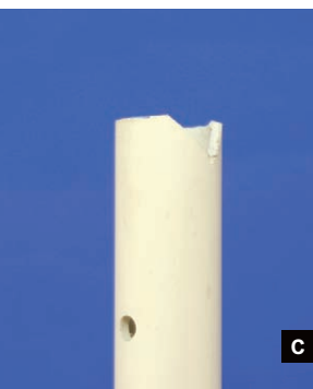
Fig. A: Materials for the light sculpture (but you can easily substitute). Fig. B: The PVC pipe frame holds a 5' PVC pipe upright. Fig. C: Notches in the top of the upright hold the main drive motor.
