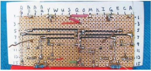
**1a.** Cut a 33×15-hole piece of perf board, then sand the edges. Scour the copper side with a Scotch-Brite pad and wipe with alcohol. Tape a cardboard frame around the edges and label the rows 1–15 and the columns A–AG, with the origin at upper left on the component (non-copper) side.
