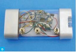
NOTE: I added the 100K pull-up resistor from power (+) to the PCB trigger to avoid EMI noise (electromagnetic interference). I also added a 0.33µF capacitor from the trigger to ground; without this, the LEDs may activate prematurely whenever the 3 switches are touched.
