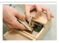
**4f.** For the other half of the lid, replace (or install) the hinges on the narrow end opposite the machine half, drilling 1/16" pilot holes.
