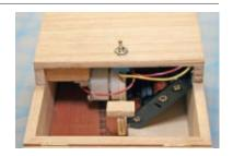
**4e.** Tweak the components' placement and the shape of the arm as needed, ungluing and regluing with hot glue, until everything does what it should. You may need to file down part of the arm so it clears the bottom of the box, or fine-tune the position of the all-important micro lever switch.
