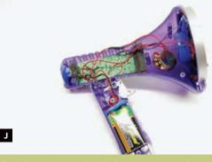
Fig. I: Another toy with a pitch control pot wired in. Fig. J: Mount the potentiometer in the housing and put it all back together.
