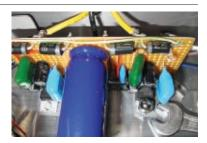
**5g.** Connect the speaker ground leads from the PCB to the black speaker terminals. Connect the speaker signal leads to the red speaker terminals, right to lower and left to upper.
