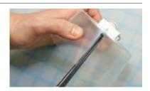
**4c.** Now put the Gyrocar together by fitting the cap over the 3 screws on the disk. Run the motor and fix the cap's position so that the gyroscope doesn't press against the track wheel constantly, but only when the Gyrocar is resting on the track wheel and the thin plastic cap flexes slightly under the gyroscope's weight.
