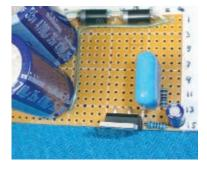
1n. Stuff and solder a 0.1µF cap into AB10 and AB14; and a 100µF into AA8 (+) and AA9 (-). On the back, bend lead AA9 down and solder it to AB13 and AA14. Bend lead AB10 up and solder it to AA8.
