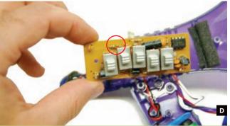
Figs. B and C: Search the circuit board for the audio generation IC, which is often a black blob "gumdrop." Fig. D: The pitch resistor is usually the resistor closest to the audio generation IC, often on the back.
