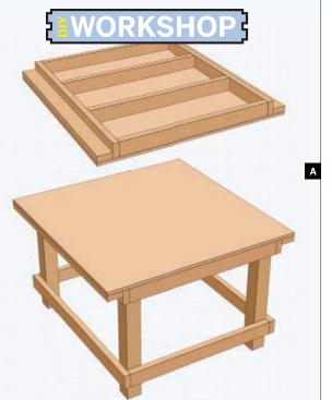
Fig. A: The tabletop is a 4'×4' sheet of <sup>3</sup>4" plywood, braced and edged with 2×4s. The table legs are 4×4s.
