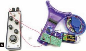
Fig. E: Replace the pitch resistor with a potentiometer of a greater value. A resistor substitution box makes the process a lot easier.
