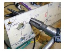
**3h.** For the square hole on part B, the input panel, you can drill a %" hole and use a 1/4" metal nibbler to cut the perimeter. Finish the hole with a flat file.
