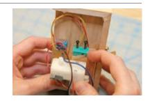
**4d.** Temporarily hold all the pieces in place with a bit of hot glue. Put the lid on the box with the other half off, load the batteries, and check to see that everything works perfectly (which is unlikely).
