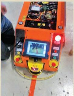
BRIGHT BOT: Archer's factory robot, called the Orange Twinkie, uses computer vision to move along a defined path and detect obstacles along the way.
