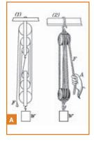
A block and tackle's ideal mechanical advantage is equal to the number of its rope segments.
