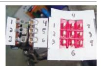
Use 3" wires to connect switch 6 to volume pot 4, switch 5 to volume pot 3 and 6 (both), and switch 4 to volume pot 1.
