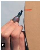
all around. Fig. D: Wrap electrical tape around the hoop joint and staples to seal against leakage. Fig. E: Mark the turntable at 60° intervals for easy placement of clamps.
