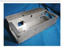
**31.** Cut \( \frac{1}{16}\)" - thick plexiglass into one piece \( 8\\\ \frac{1}{2}\)" \( 2\\\ \frac{1}{6}\)" (for the top) and 2 pieces \( 2\\\ \frac{1}{2}\)" \( \frac{1}{2}\)" (for the sides). Notch out the lower corners of the side pieces so they clear the nuts in the D rails. Test-fit these pieces and trim to fit
