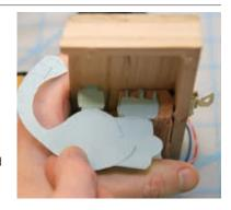
**2c.** Mark the positions on the templates where they meet: the toggle and bracket's position on the lid, and the motor and switch's position on the bracket.
