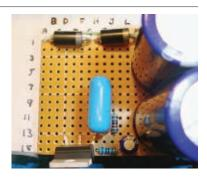
1i. Stuff and solder a 0.1µF cap into G10, G14; and a 100µF cap into F8 (+), F9 (-). On the back, bend lead F9 down and solder it to F13 and G14. Bend lead G10 up and solder it to F8. Clip the other leads, except for F8.
