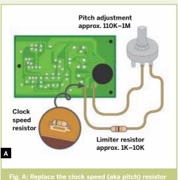
Fig. A: Replace the clock speed (aka pitch) resistor with a potentiometer and a limiting resistor.
