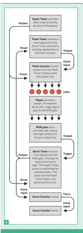
Fig. A: This block diagram shows how the components interact.
