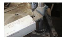
**3f.** For larger holes, drill a small hole first to make the bit easier to center. You can also cut large holes with a step bit (aka castle bit or unibit).
