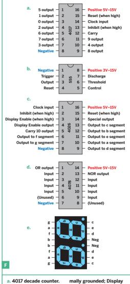
Reset and Inhibit pins are normally grounded.
