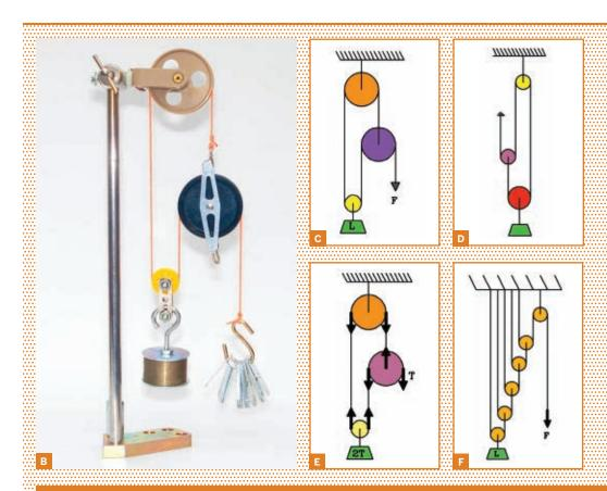
PITY THE FOOL: Fig. A: (Opposite page) A typical block and tackle. Fig. B: The fool's tackle. A pulley system can't physically exist in this configuration; it collapses immediately. This one is stopped by a wedge of foam plastic between the top pulley and its frame. (Call it a "blocked tackle"?) Fig. C: The classic fool's tackle. Fig. D: An inverted fool's tackle. Fig. E: Force analysis of the fool's tackle. Fig. F: The Spanish burton.
