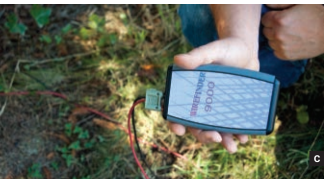
Fig. A: The completed WireFinder transmitter in a sleek project enclosure. Fig. B: The completed transmitter, opened up to show component placement. Fig. C: Connect the buried wire or cable directly to the
