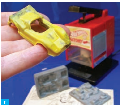
DESKTOP GARAGE: Figs. R and S: Kenner's 1962 Motorized Home Workshop promised "planes that fly and boats that float" but the flimsy foam made fuzzy and feeble results. Fig. T: Mattel's 1969 Injector had a hand-powered injector piston for molding hot plastic. Figs. U and V: The Hasbro Kid and Matty Mattel — these sworn rivals vied to rule the maker toy market.
