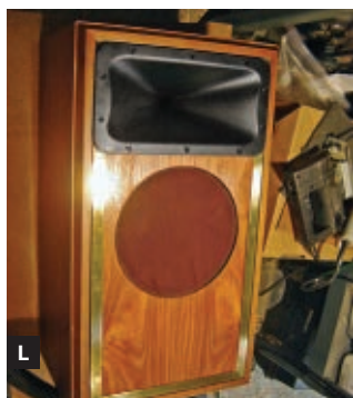
Fig. J: Finished speaker. Fig. K: Finished speaker with new grille. Fig. L: An alternate version, with back-mounted woofer and a fancy finish, including a new veneered baffle board with brass trim.
