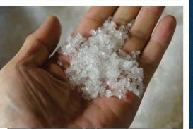
once 3% saltwater has become *nigari* (bittern), the coagulant used for making tofu, with a salt content of 23 to 32%. The final step involves a small centrifuge resembling a washing machine. Each day Nakamichi-san packs the harvested salt in net bags and sets them on the spin cycle to remove excess moisture.
